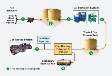
When a fuel arrives on site, it has gone through production, storage, transport and storage. Few fuels are so clean after this cycle that that they can be used without treatment. Analysis requirements start with the delivery of the fuel, continue throughout fuel handling, and end only as the fuel is injected into the turbine. Preconditioning of the fuel before it reaches the gas turbine is a prerequisite for installation when contamination may be present.
